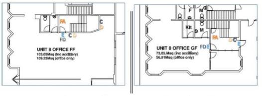
CM Alarm SA Fire Door FD CO2 Extinguisher C Dry Powder Extinguisher D EXIT 🔋 Alarm 🤼
